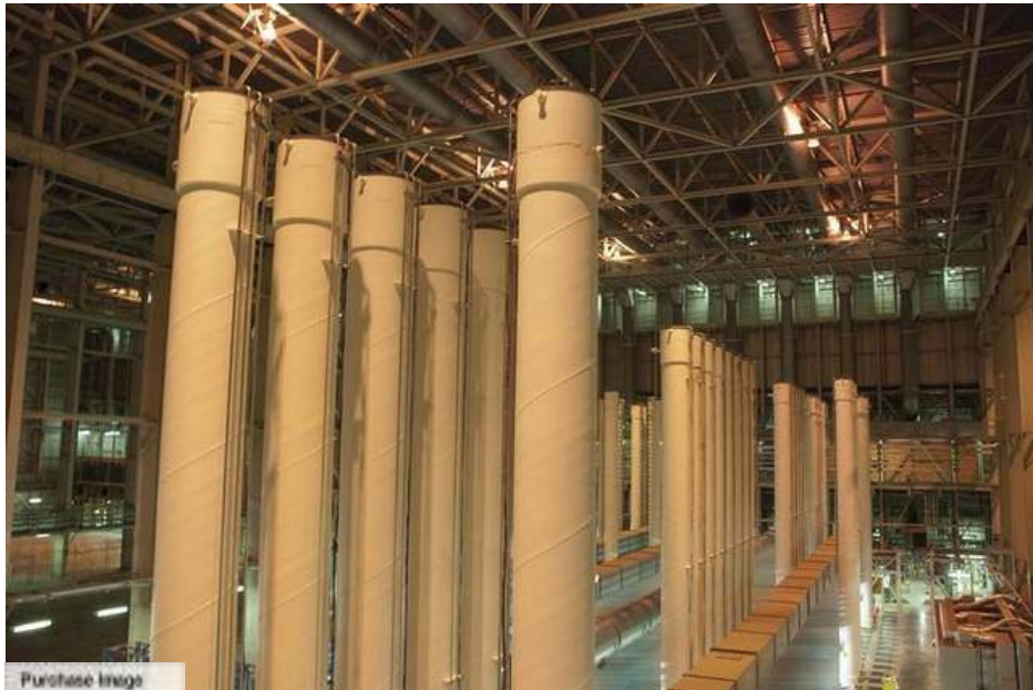
This 2010 photo shows a series of AC100 centrifuge machines at the American Centrifuge Plant. The centrifuge project has become the center of attention in the debate about whether the Department of Energy is being pressured to push loan guarantees through too quickly. / Gazette file photo
