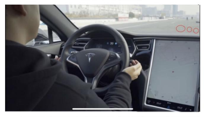
In-car perspective when testing, the red circle marks, the interference markings are marked with red circles
