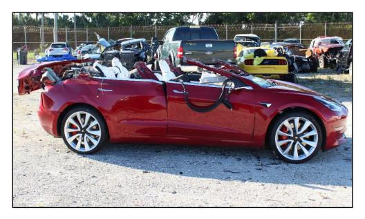
Figure 2. Tesla Model 3 with extensive roof damage photographed postcrash at tow yard.
